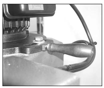
Figure 14. Belt adjustment handle.
